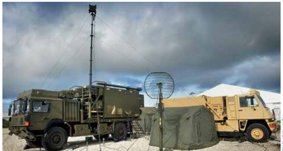
An early entry small form factor palletised version of the Falcon area communications system, shown here on exercise with HQ Allied Rapid Reaction Corps (ARRC), has been developed to provide a rapidly deployable capability. It is expected to be introduced by the end of 2017.
